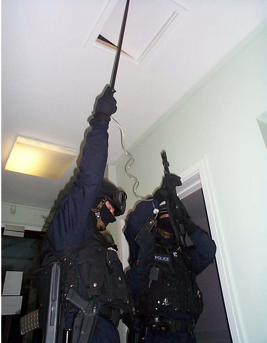
Goodman Bentley Gas Data Stowcheck Co2 Loft probe seen being used to analyse a loft space for a hidden person
